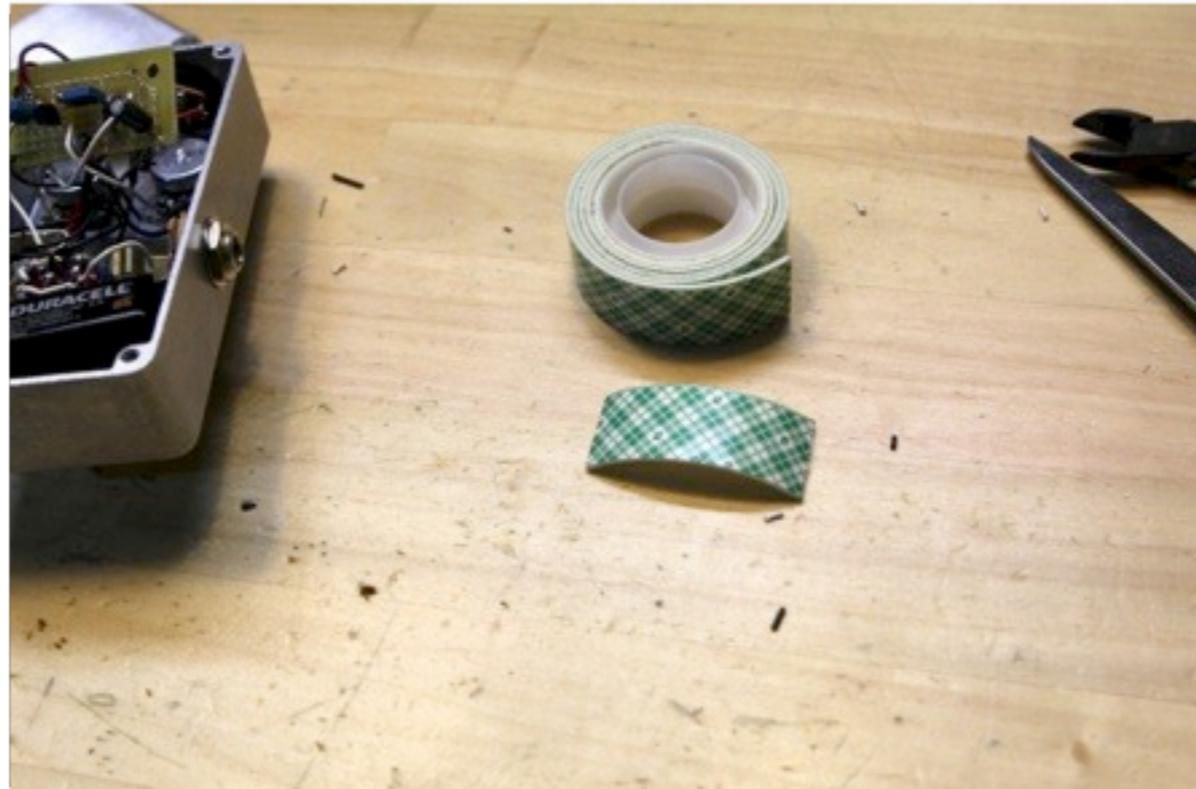
Fasten the perfboard assembly to the back of the tone pots, preferably using a short length of double-sided foam tape. This will keep the components in place and prevent any perfboard components from shorting out from contact with the pots.
